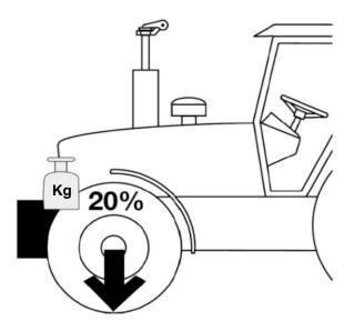
Figure 4. Minimum front-axle load of the tractor
