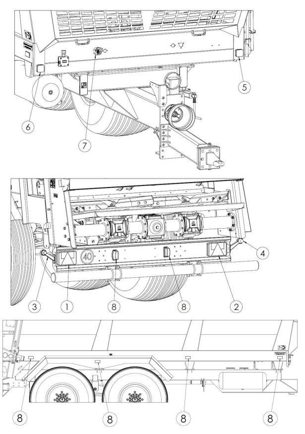
Figure 15. Arrangement of the electrical system components: 1 – rear left lamp cluster, 2 – rear right lamp cluster, 3 – left marker light, 4 – right marker light, 5 - front left running light, 6 - front right running light, 7 - connection socket, 8 reflector
