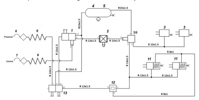
Figure 12. 2-line pneumatic braking system with ALB
