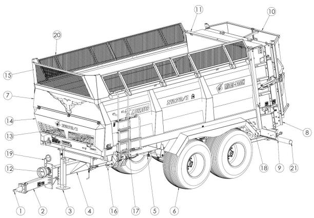
**Figure 8.** General design of the Manure Spreader:
