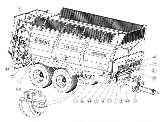
Figure 5. Layout of warning and information decals on the vertical adapter (front)
