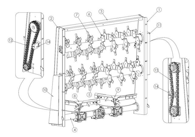
Figure 11. 2-auger horizontal disc adapter
