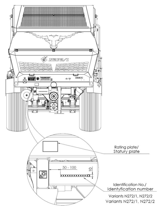
Figure 3. The location of the rating plate and the VIN number
