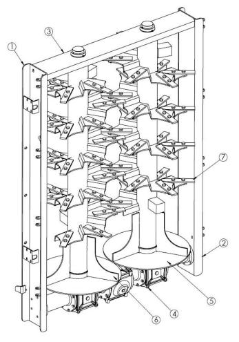
Figure 9. 2-rotor verticaladapter
