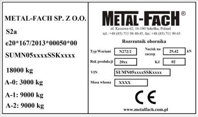
Figure 1. Rating plate and VIN number
